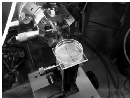
Fig.2 The glass capillary at the end of beamline inserted in a liquid container.
