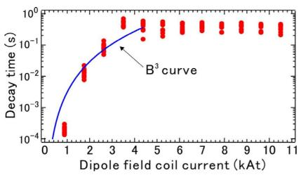
τ in the variation of magnetic field strength B (at the base pressure of B=5 × 10<sup>-7</sup> Torr)
