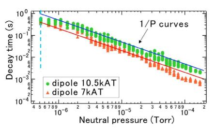
$\underline{\tau}$  in the variation of the back pressure P (addition of hydrogen gas, in the dipole field of  $l_{ic}$ =7kAT)
