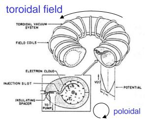
1950~ Toroidal electron plasma in a pure toroidal field
