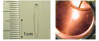
Probe filament and electron emission
