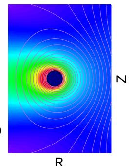
Example of magnetic surfaces (thin lines) and field strength
