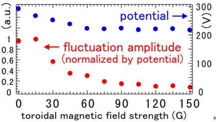
Amplitude of the electrostatic fluctuation in the diocotron frequency range is stabilized, while the generated plasma potential is approximately constant.
