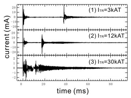
When a toroidal field is added, the plasma tend to disrupt during the trap phase.
