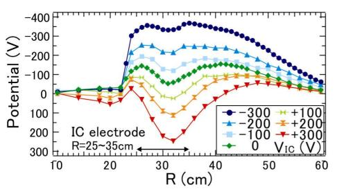
Radial potential profiles at Z=+6cm in the variation of bias voltage of the IC electrode (Vic)
