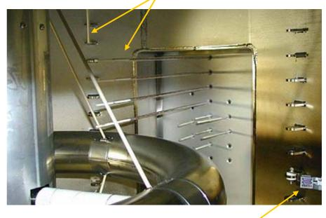
Internal conductor (IC) (dipole field coil) and electrode
