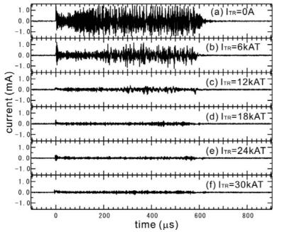
Stabilization of diocotron mode by the addition of (magnetic shear) toroidal field\*
