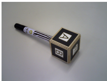
Figure 4: The AR pen: A cube composed of five AR markers is attached at the end of a pen.
