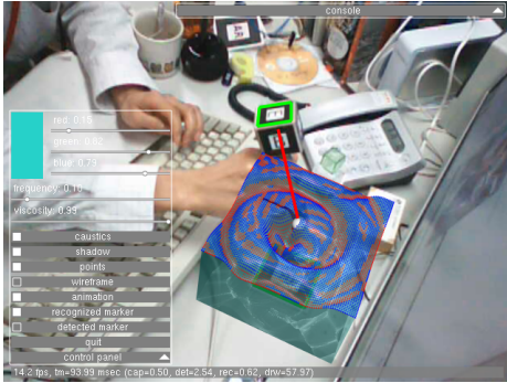
Figure 7: Visualization of acceleration. Red points show upward acceleration and blue points show downward one.
