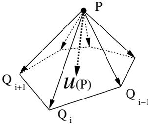
**Figure 2. Umbrella operator associated with a mesh vertex  $\mathbf{P}$  is defined as a weighted average of the neighbor vectors, see (2.4).**
