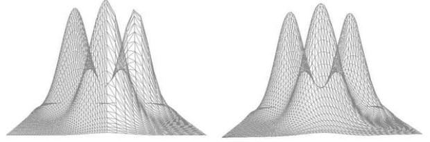
**Figure 3. Left: a mesh consisted of two parts with different sampling rates. Right: tangential mesh evolution (2.3) with  $\tau^{(k)} = 0$ , (2.5) was used to equalize the mesh triangles.**
