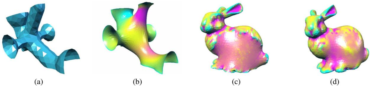
**Figure 1. Generating fair triangle meshes with discrete elastica. (a) An initial mesh outlined a complex tubular object. (b) A discrete elastica surface (mesh) obtained from the initial mesh. (c) The Stanford bunny model with a large part of the mesh removed and then triangulated. (d) The modified part of the bunny is restored as a discrete elastica. Coloring by the mean curvature is used to demonstrate a high quality of the generated meshes.**
