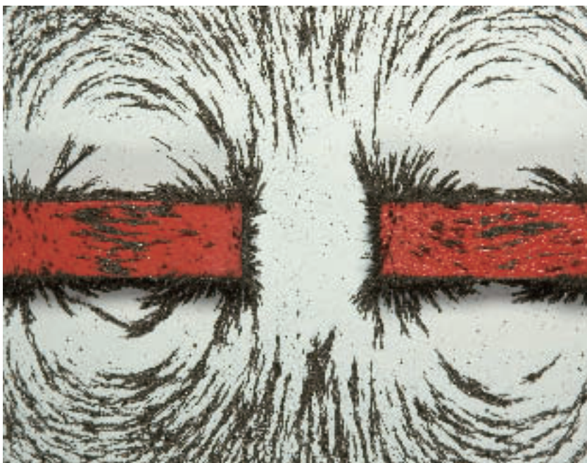
Figure 1: Charged particle spins of a bar magnet generate a magnetic field.
