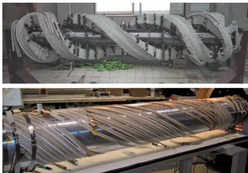
Figure 1: Helically twisted magnets from the newly installed warm conducting (top) and cold superconducting (bottom) Siberian snake devices in the Alternating Gradient Synchrotron at Brookhaven National Laboratory.
