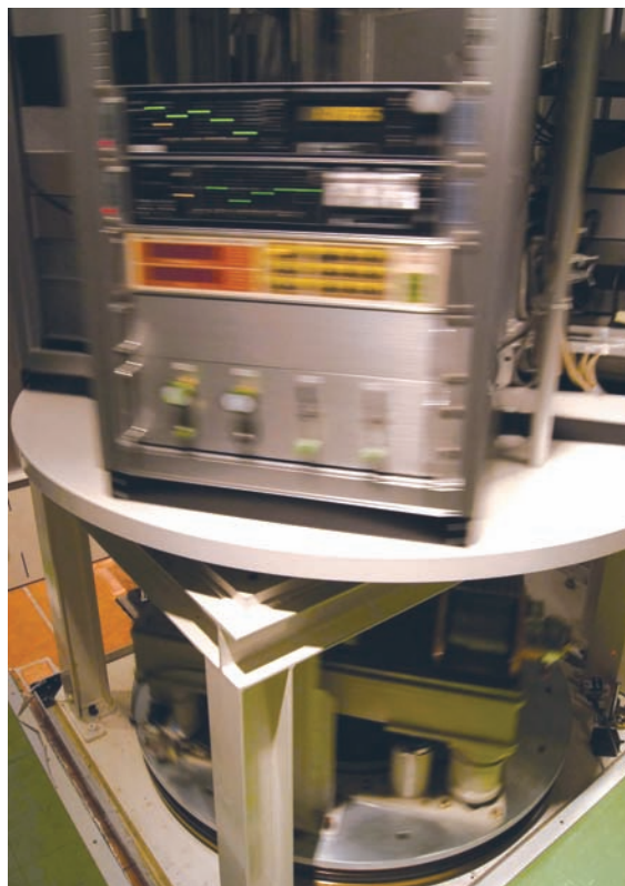
Figure 1: A custom-developed rotating cryostat capable of 15 millikelvin temperatures is helping physicists find evidence for the existence of supersolids.
