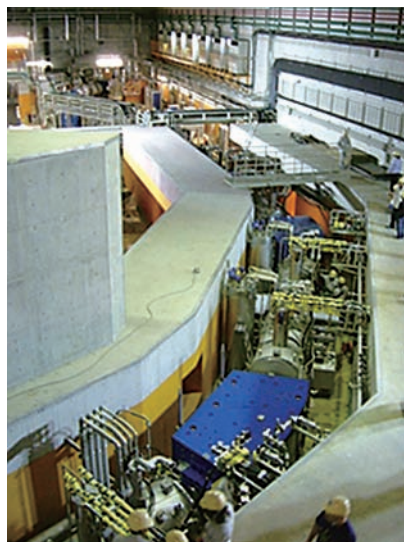
Figure 2: The first stage of the BigRIPS separator at the RIBF uses superconducting magnets to sort short-lived isotopes by mass and charge.
