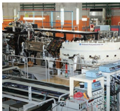
Figure 5: The SCRIT-based radioisotope-electron scattering system under development and preliminary operation.
