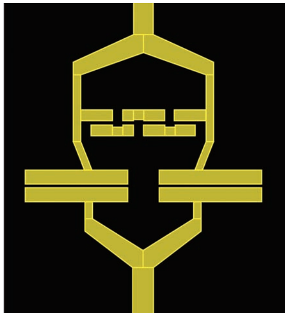
Figure 1: Layout of the superconducting flux qubit, which consists of several aluminum circuits. The key elements are the three 'islands' of metal in the top half of the image, across which the superconducting current flows. Magnetic pulses applied to the qubit control its quantum states.
