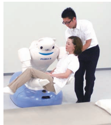
RIBA-II can now lift a person from floor level
