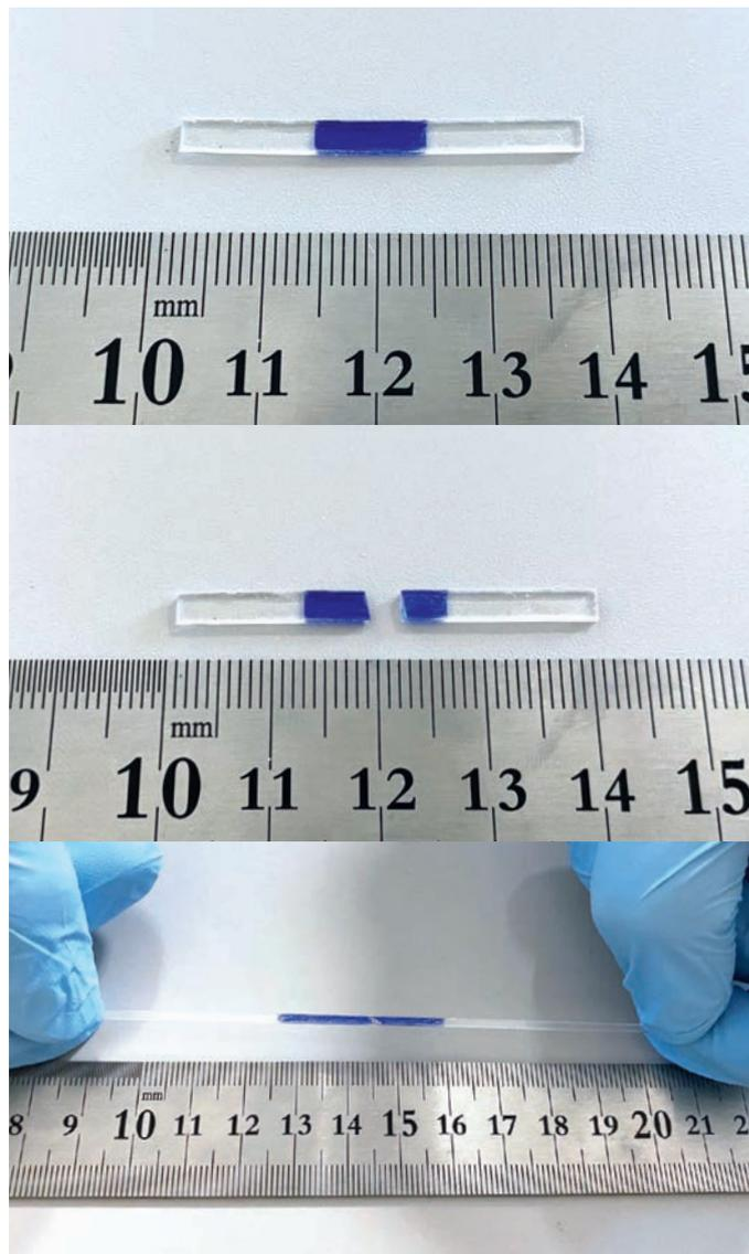
A sample of self-healing polyisoprene (top) was cut into two pieces (middle) and then pressed together for 15 seconds. After one minute, the sample could be stretched to more than double its original length without breaking (bottom).
