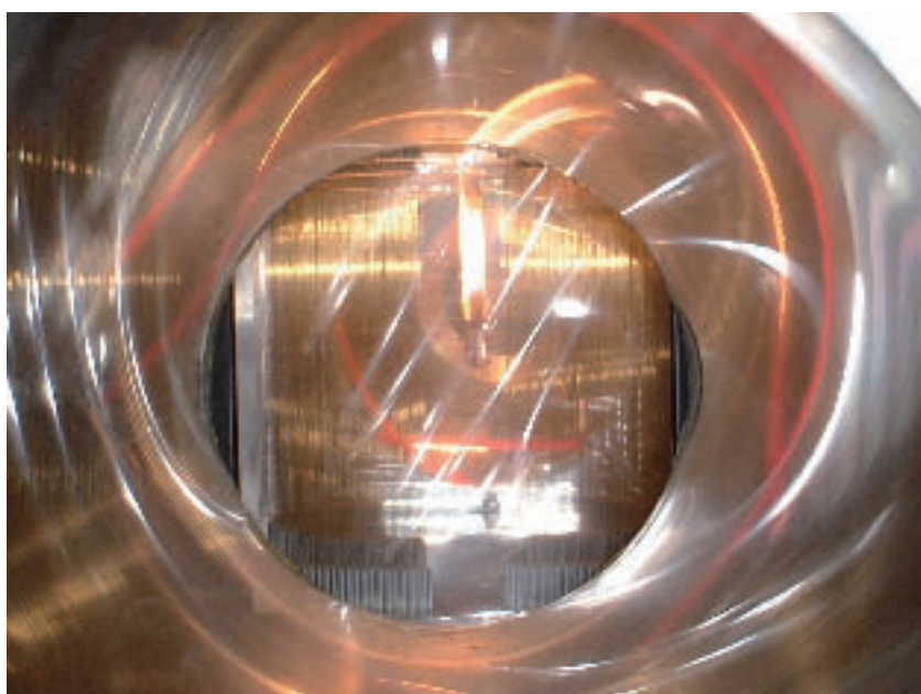
Figure 1: A view inside the spectrometer to detect the decay products of vector mesons. The centre of the image shows the small copper target where the \phi mesons are produced by incident protons. The structures around the target are the detectors for the meson decay products.
