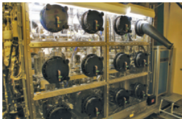
Facility for preparing tritium and deuterium samples for muon-catalyzed nuclear fusion in the RIKEN-RAL Muon Facility
