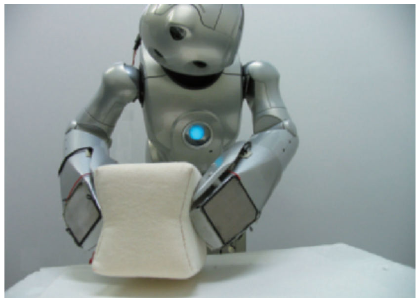
Figure 1: A humanoid robot executes one of its tasks, which involves picking up an object, shaking it side to side three times, and setting it back down. Use of the robot was made possible through a collaboration with SONY Corporation.
