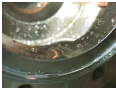
Figure 3: Photograph of a flood in a vacuum chamber after the liquid cell window breaks.
