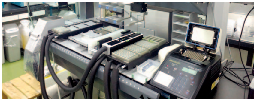
Figure 1: The automated CAGE cDNA preparation system for rapid genome-wide gene expression analysis.
