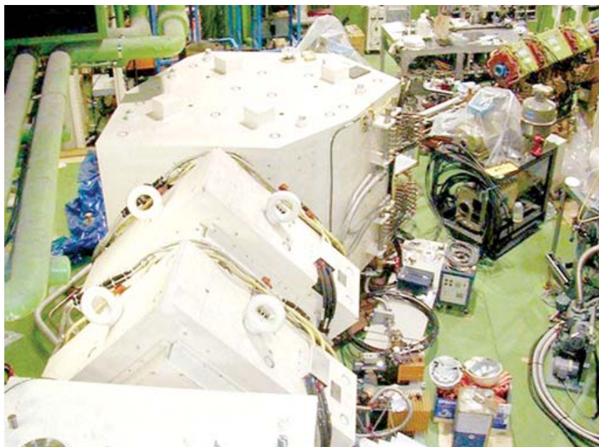
Figure 2: The Gas-filled Recoil Ion Separator (GARIS) separates the nucleus of element 113 from any unwanted ions and directs the nucleus into a detector chamber.
