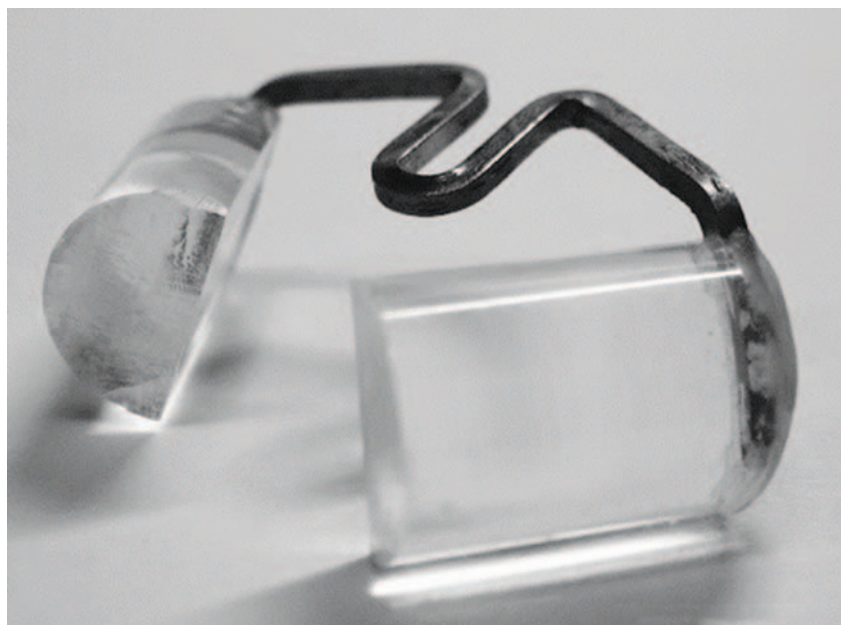
Figure 1: Specially designed goggles modify visual input so that only vertically oriented stimuli are perceived.
