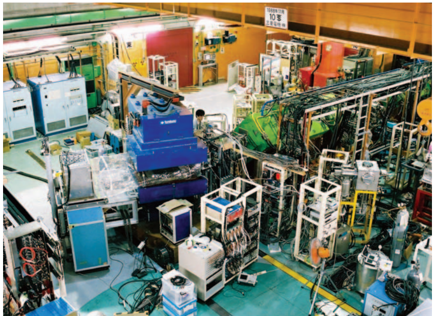
Figure 1: The RIKEN Projectile fragment Separator (RIPS) (pictured) produces high-intensity beams of radioactive ions, which help scientists in the study of nuclear processes.
