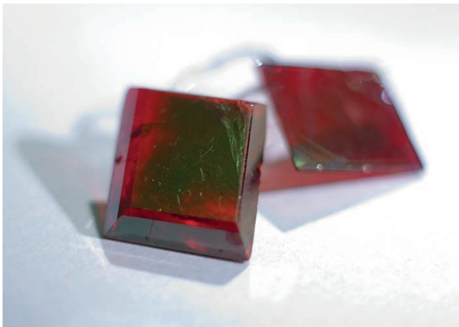
Researchers at the RIKEN Terahertz-wave Research Group use nonlinear optical crystals to produce intense laser beams with terahertz frequencies (above and opposite page).
