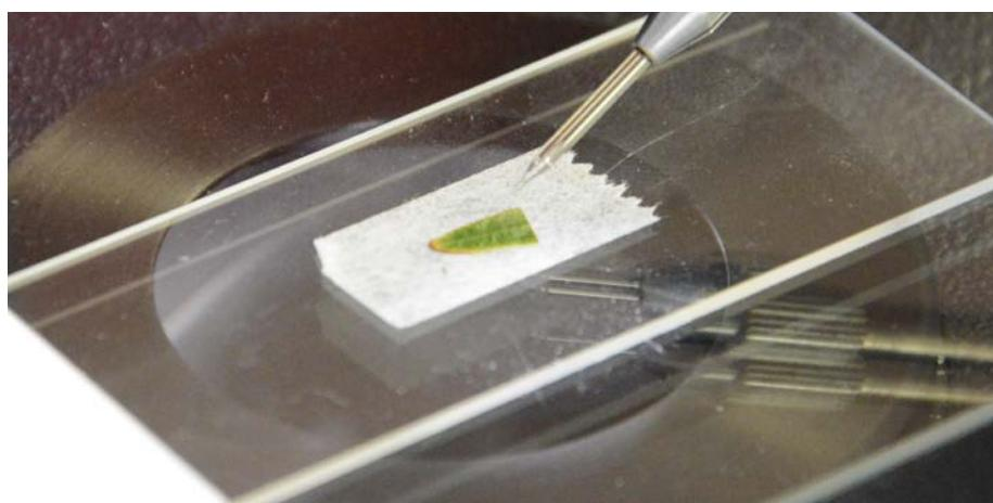
A nanospray tip is used to extract the contents of a single plant cell, which are then analyzed by a mass spectrometer, providing a rapid analysis of the molecular contents of the cell.
