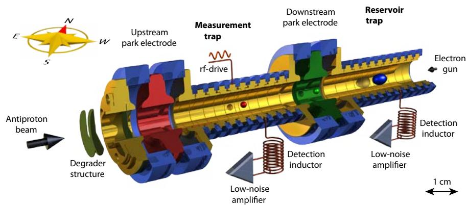
Schematic of a magnetic Penning trap at the Antiproton Decelerator in CERN (European Organization for Nuclear Research).
