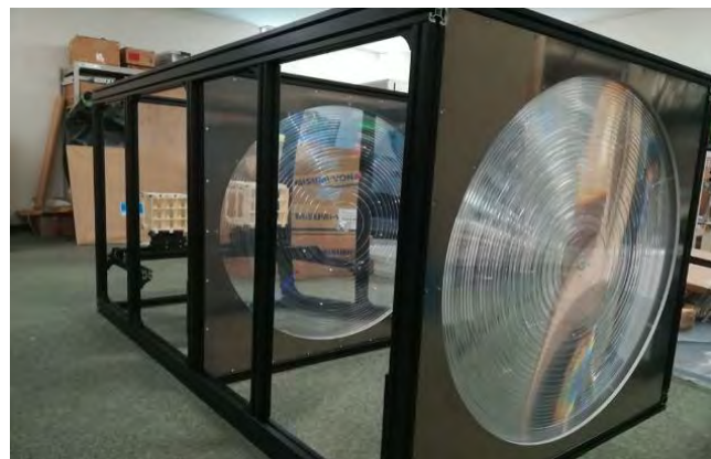
Figure: The drawing of the wide field telescope (left) and that manufacture (right).
