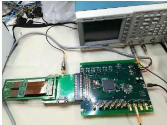
Figure 2 : Dedicated analog to digital conversion board for 128 channels (left) and the test bench (right)
