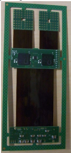
Figure 2 : Dedicated analog to digital conversion board for 128 channels (left) and the test bench (right)
