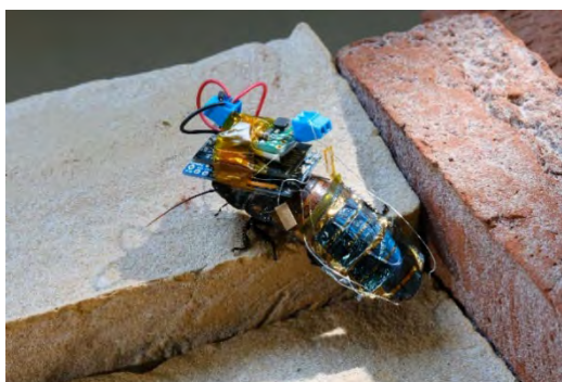
Figure 1. Rechargeable Cyborg Insects using ultrathin organic solar cells
