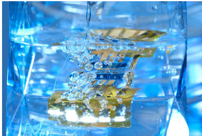
Figure 1. Ultra-Thin Organic Solar Cell Capable of Long-Term Operation Underwater
