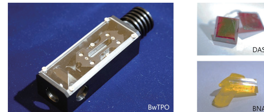
Backward terahertz parametric oscillator (left) and organic nonlinear crystals (right)
