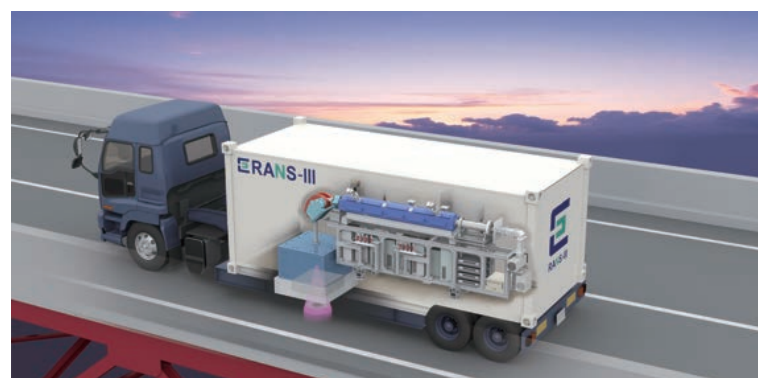
The future imaging of compact neutron non-destructive test system on-site
