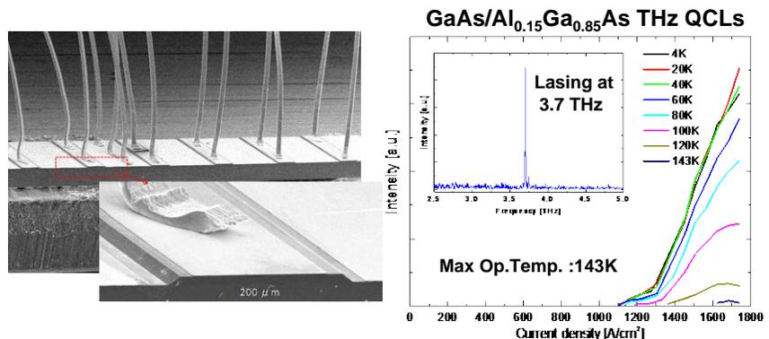
Fig. 4. Achievements of high-temperature operation of GaAs-based THz-QCLs
