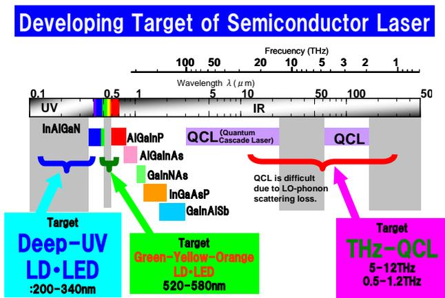
Fig. 1. Development target for new-frequency semiconductor light-emitting devices
